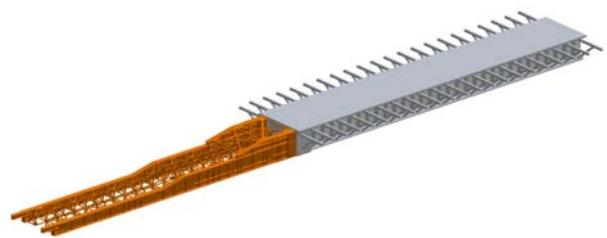
Fig. 4. Incremental launching using the core section
