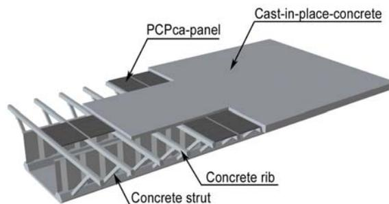
Fig. 5. Construction method of upper slab
