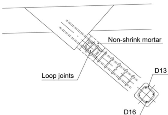
Fig. 10. Upper joint of the strut
