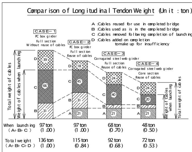
Fig. 8. Comparison of longitudinal tendon weight
