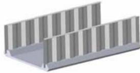
STEP-2 Erection of ribs and struts. Placement of PCPca panels at the core section upper slab (in main girder fabrication yard)
