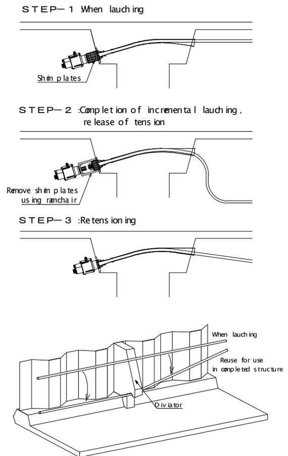
**Fig. 7.** Diverting of the temporary erection cables
