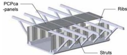
STEP-3 Placement of concrete at the core section upper slab, Tensioning of PC cables (in main girder fabrication yard)
