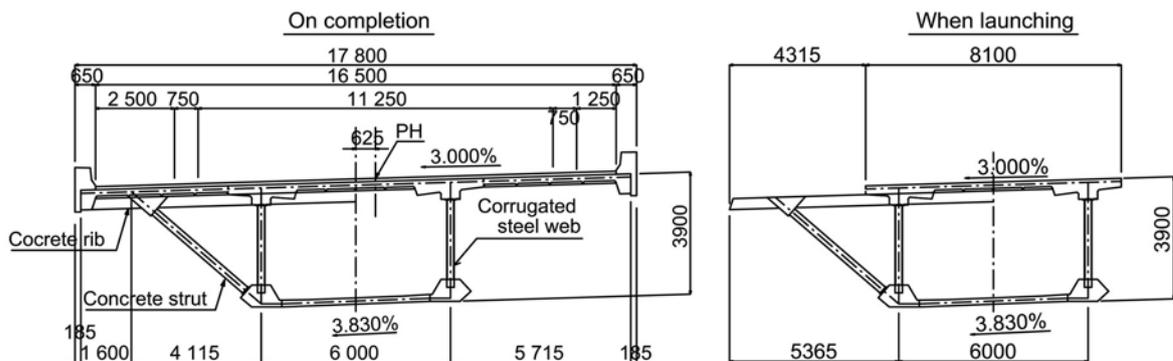
Fig. 2. Cross section
