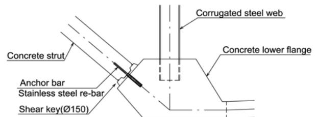
Fig. 11. Lower joint of the strut
