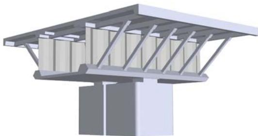
Fig. 3. Corrugated steel web box girder structure with ribs and struts
