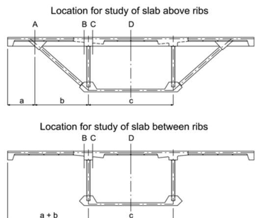
Fig. 9. Location for study of slab with ribs and struts
