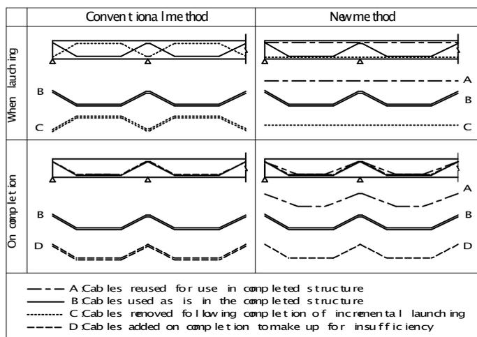
Fig. 6. Layout of the prestressing cables
