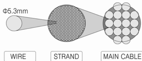
Figure 14. Cross Section of Main Cable
