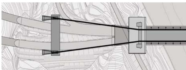
Figure11. 3-Dimensional Cable of Side Span
