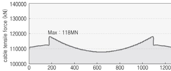
Figure 5. The Cable force of Inclined Pylon
