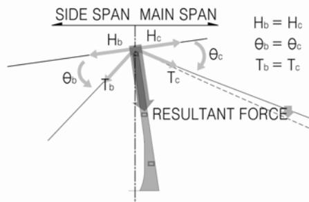
Figure 3. The Principle of Inclined Pylon
