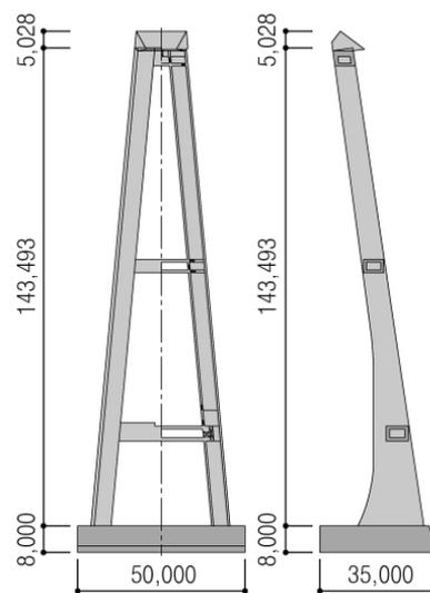
Figure 9. General View of Inclined Pylon
