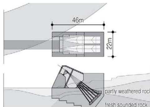
Figure 19. Gravity Anchorage System
