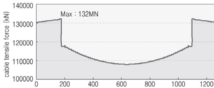
Figure 6. The Cable force of Perpendicular Pylon
