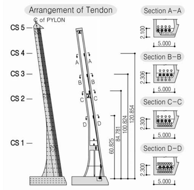
Figure10. Construction Stage of Inclined Pylon
