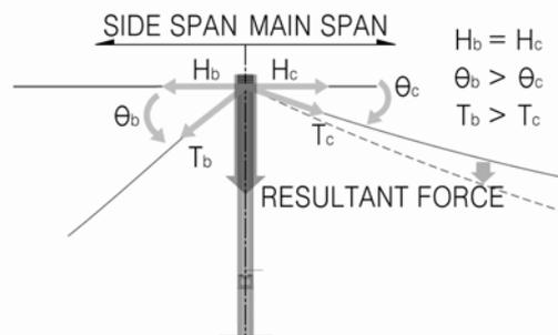
Figure 4. The Principle of Perpendicular Pylon
