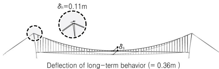
Figure 7. The Displacements of Inclined Pylon
