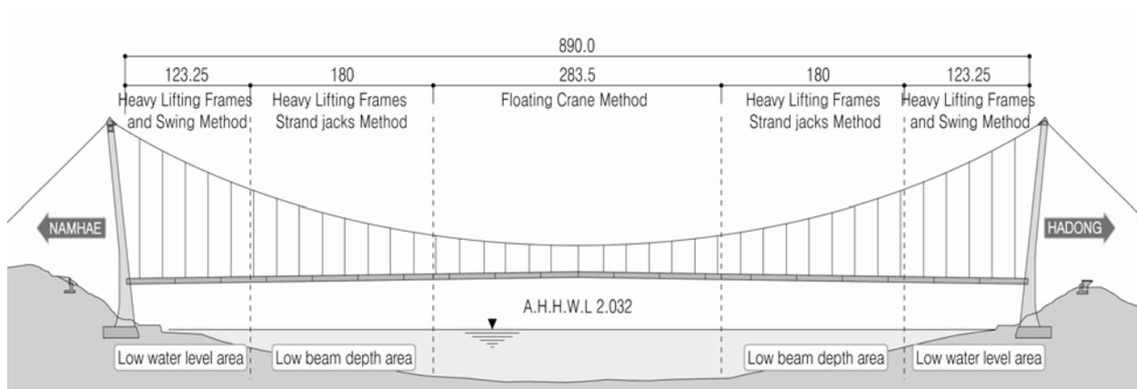
Figure 20. Erection of Stiffening Girder
