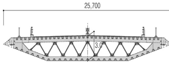
Figure 16. Streamline-Shaped Stiffening Girder
