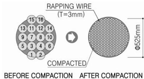
Figure 15. Compaction of Cable
