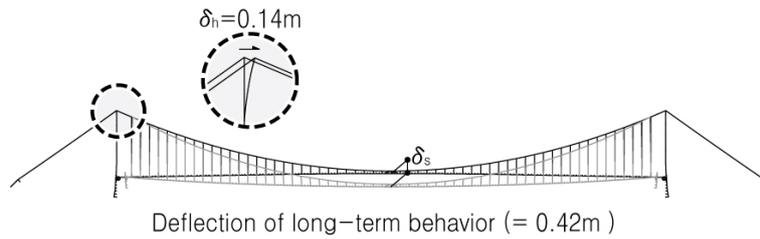
Figure 8. The Displacements of Perpendicular Pylon
